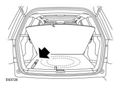
Storage position for a warning triangle is located on the left-hand side of the under-floor storage area.
